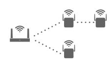
**Extension of streaming range** via additional repeater installation
