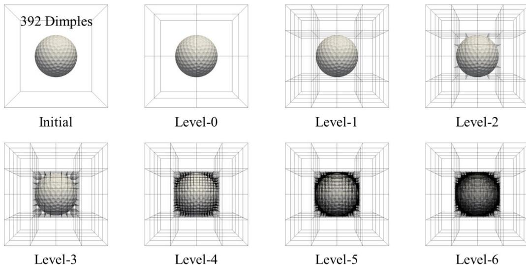
Figure 1. Adaptive mesh refinement procedure (level-0 to 6) for computing signed distance function of a golf ball
