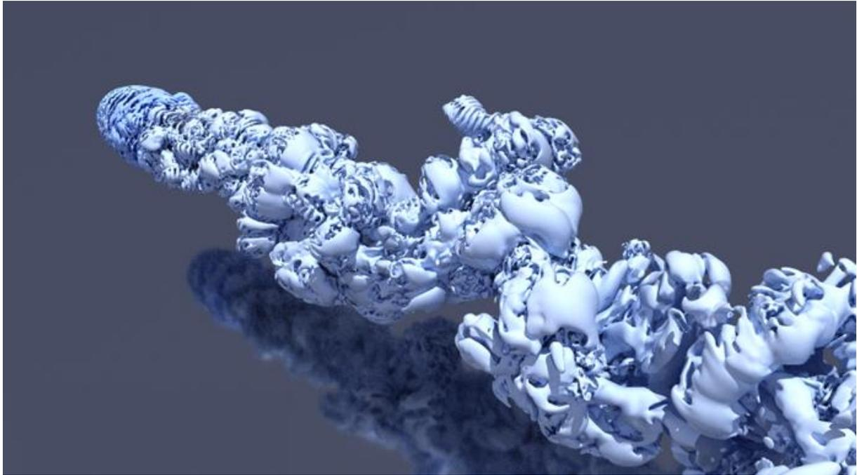
Figure 2. Instantaneous vortical structure based on  $\lambda_2$ -definition behind a stationary golf ball at  $Re = 1.1 \times 10^5$
