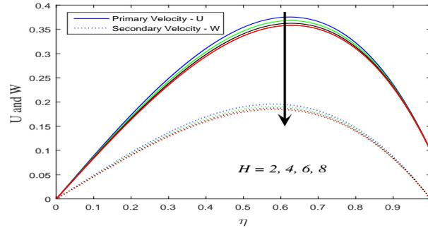
FIGURE 12. Influence of  $H$  on fluid primary velocity and secondary velocity.
