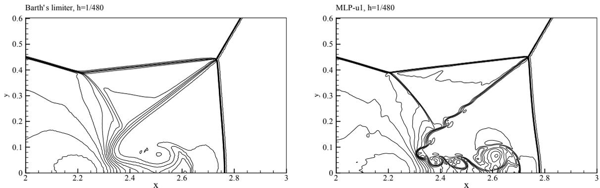
Figure 2. Density contours around the region of the double Mach stem
