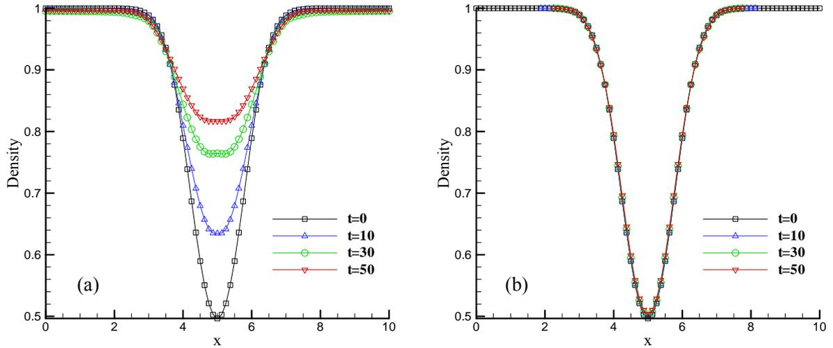
Figure 1. Density distributions along the vortex center: (a) Barth's limiter and (b) MLP-u1
