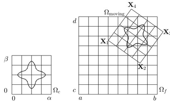
Figure 1. Schematic illustration of the fluid domain  $\Omega_f$ , the crystal domain  $\Omega_c$ , and the moving domain  $\Omega_{\text{moving}}$ .
